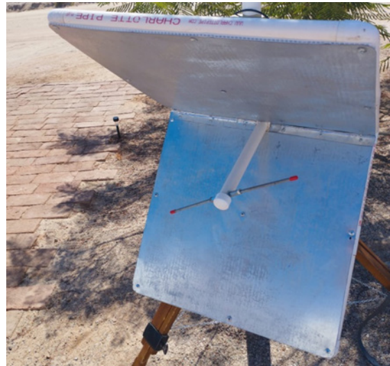
Figure 7C – The metallic reflector glued and screwed to the Plaskolite.
