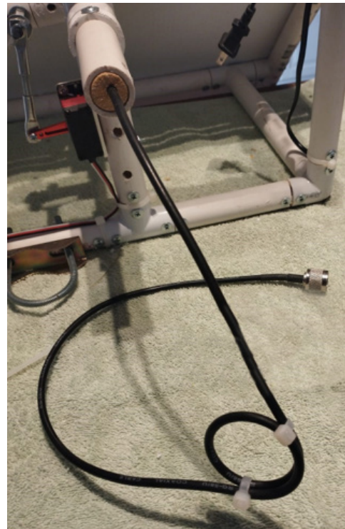
Figure 9 – This air-wound, common mode choke is made of 1.9 turns of RG8X coax with a diameter of 40 mm. The RF choke must be tuned. See text.
