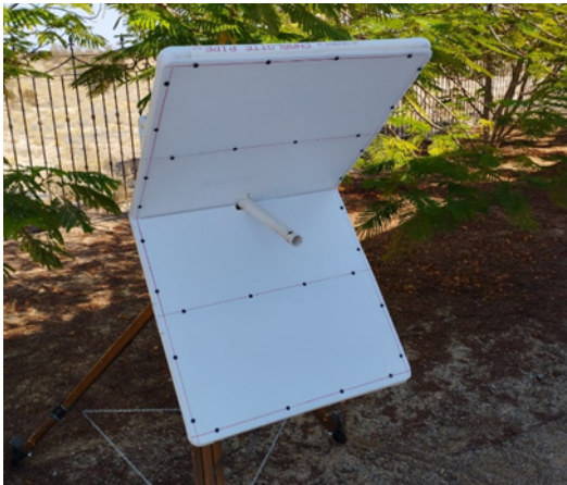
Figure 7B – The antenna PVC frame with the Plaskolite corrugated plastic applied.
